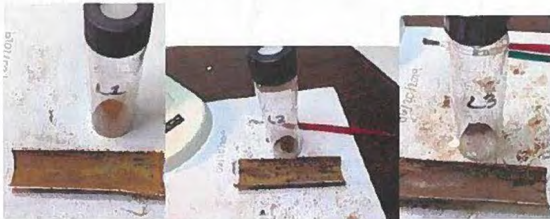
Figure 4-13 Layers of Scale Removed from Harvested Pipe
