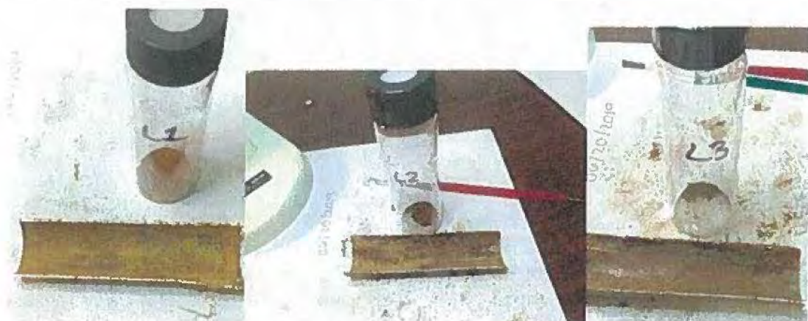
Figure 4-13 Layers of Scale Removed from Harvested Pipe
