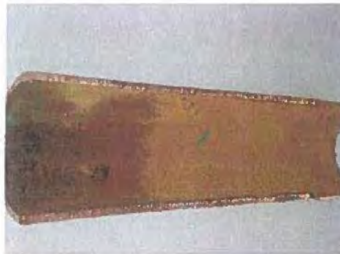
Figure 4-12 Pipe Prior to Scale Removal
